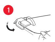
Spool off enough thread. Hold upper thread at the reel and thread with other hand. Slip thread under top thread auide.
