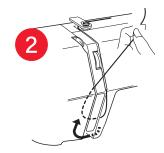
Guide thread down right channel and around the bottom of the thread guide plate. Pull firmly to ensure thread slots into tension disks.
