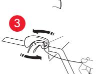
Firmly, draw thread up left channel and into the thread take-up lever.
